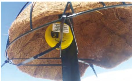
Tinytags were used during the trials to monitor the temperatures outside and inside the silo bags.
