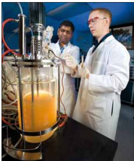
Chemist Badal Saha and technician Greg Kennedy collect a sample of a fungal culture to determine whether fermentation inhibitors are present after the pretreatment of wheat straw feedstock. Inhibitors can stop or reduce the rate of ethanol fermentation. (PHOTO: Stephen Ausmus)
