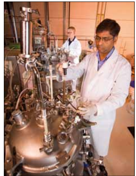
Technician Greg Kennedy (left) and chemist Badal Saha sample cellulosic ethanol from wheat straw produced in a 100-litre fermenter to assess its ethanol content and to monitor how quickly the sugars in the wheat straw are being fermented into ethanol. Using the 100-litre fermenter allows the scientists to scale up the process so that they can finetune it and identify technical problems that might develop during large-scale ethanol production.
