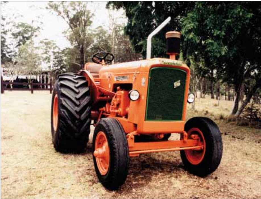
Pictured is the Chamberlain Super 90 again, clearly showing the soft riding transverse leaf spring front suspension. The tank alongside the engine is in fact the hydraulic reservoir to which is attached the valve control block. In an endeavour to deflect the roar of the two stroke engine, in this example the exhaust pipe has been extended and angled away from the operator. On a still evening, when night ploughing, the distinctive sound of a Super 90 under power could be heard for miles. (PHOTO: IMU)
