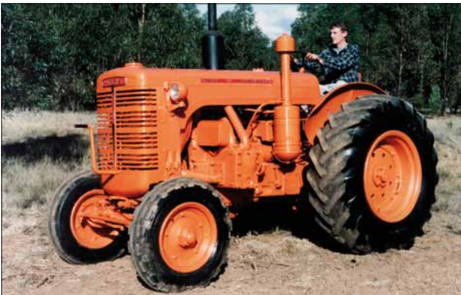
Mathew Puls of Dubbo, NSW is seen here demonstrating his immaculately restored Chamberlain 40KA. Note the horizontally opposed twin cylinder engine which was designed to run on power kerosene fuel, following its initial start on petrol. (PHOTO: IMJ)
