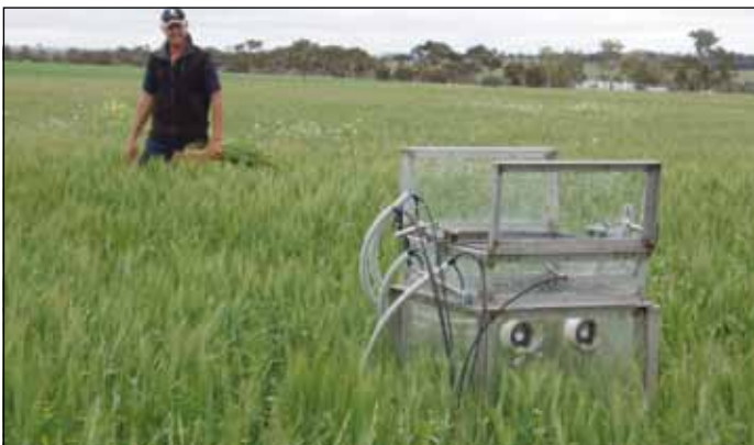
UWA Research Associate Dr Andrew Wherrett collecting plant samples at DAFWA's Wongan Hills Field Research Station, with a chamber used for measuring in-situ nitrous oxide emissions in the foreground.
