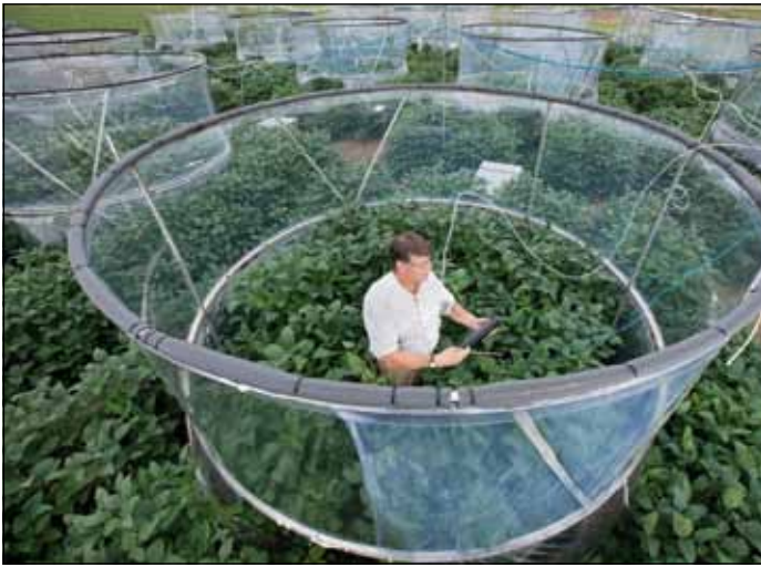
Plant physiologist Fitzgerald Booker prepares to place an optical scanner into a tube that will be positioned in the soil to photograph soybean roots. The photos will be analysed to determine changes in root length and distribution caused by exposure to elevated carbon dioxide and ozone, which are pumped into the open-top field chambers. (PHOTO: Peggy Greb)
