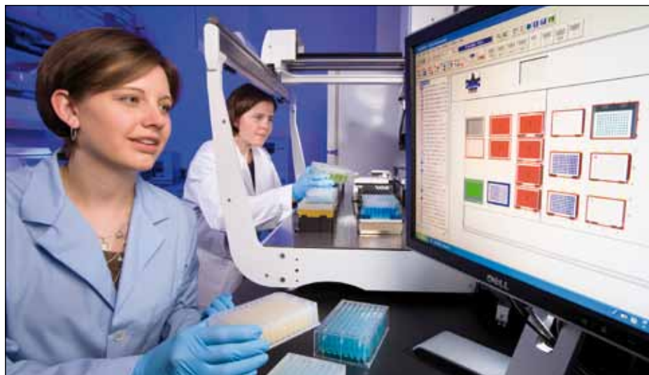
To assess oxidative stress in soybean grown at SoyFACE under elevated ozone concentrations, ARS molecular biologist Lisa Ainsworth (back) and graduate student Kelly Gillespie use a liquid-handling robot to perform a high-throughput assay. (PHOTO: Peggy Greb)
