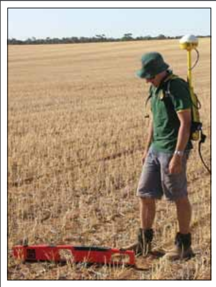
EM38 mapping at Carwarp in Victoria's Mallee.
