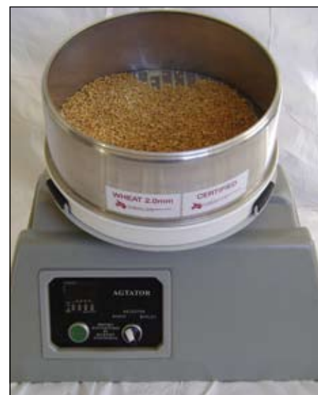
The Agtator automates the shaking action to analyse screenings. (Photo: Craig Moore)
