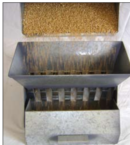
Grain dividers accurately split samples into representative sub samples. (Photo: Craig Moore)
