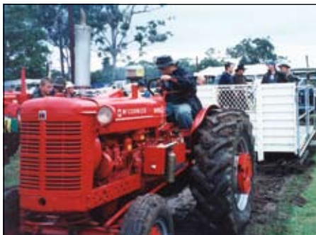
An International McCormick WD6 is fitted with axle weights which extend wider than the rear wheels. At some tractor pulls this would be disallowed. (Photo M. Pettit)
