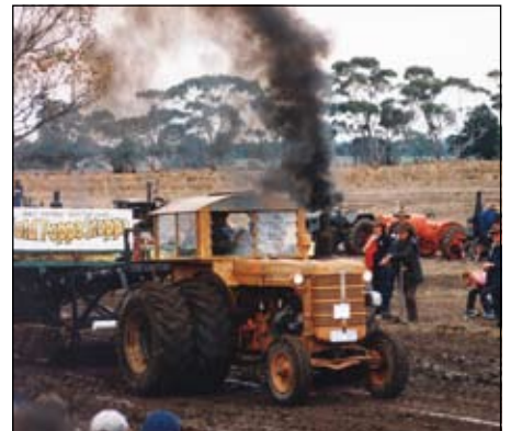
This poor old Chamberlain has been repowered with a doctored 100 hp engine and fitted with dual rears. (Photo IMJ)
