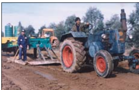
This Lanz Bulldog is equipped with standard cast iron rims. What is not noticeable is the fact that the sheet metal floor of the cockpit has been replaced with three inch cast steel. (Photo C. Galbraith)
