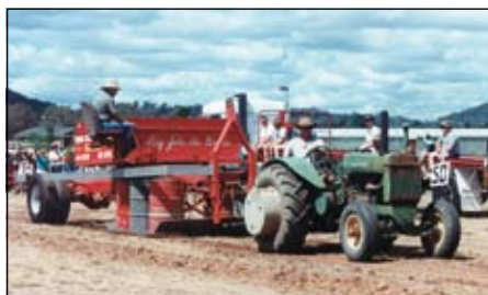
A John Deere AR with grossly heavy concrete counterweights attached to the rear wheels. (Photo IMJ)
