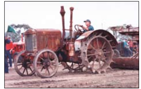
This old McCormick is equipped with steel wheels and lugs. People often mistakenly assume that these lugged wheels will obtain greater traction than if fitted with pneumatic tyres. Nebraska Tractor Test figures prove that in fact the pneumatics obtain a greater grip of the ground. (Photo IMJ)
