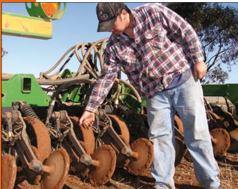
David Mclagan points out a problem their soils can cause when ‘sticky’. The mud can collect within the gauge wheel and stall the disc.
