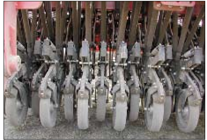
Disc seeders were cited as well suited to narrow row spacing requirements such as for pasture establishment and renovation.
