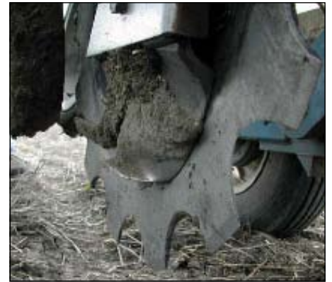
Low soil disturbance attributes of disc seeders were seen to minimise seedbed moisture loss, reduce weed pressure and improve crop establishment in marginal moisture conditions.
