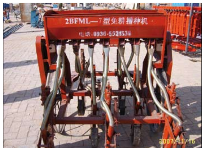
This Chinese generation II prototype zero till planter was developed from Australian and overseas bed planters by Dr Jack McHugh and interpreted by local engineers in the Hexi Corridor of NW China. Implement cost, mass, and depth control were key concerns.
