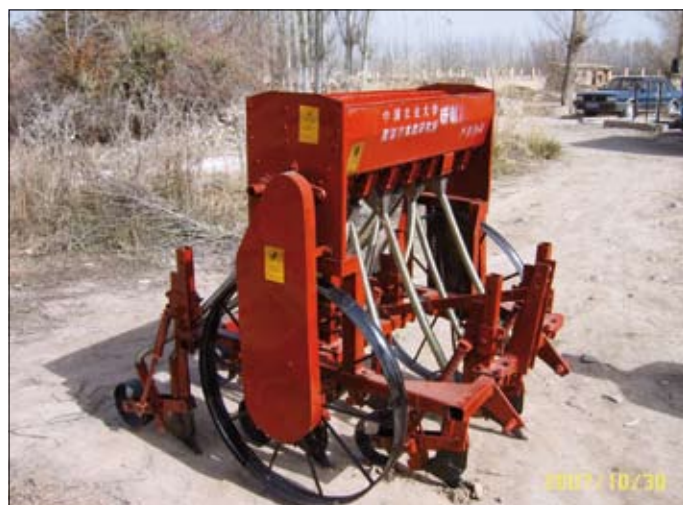
This Chinese generation II prototype zero till planter was developed from Australian and overseas bed planters by Dr Jack McHugh and interpreted by local engineers in the Hexi Corridor of NW China. Implement cost, mass, and depth control were key concerns.
