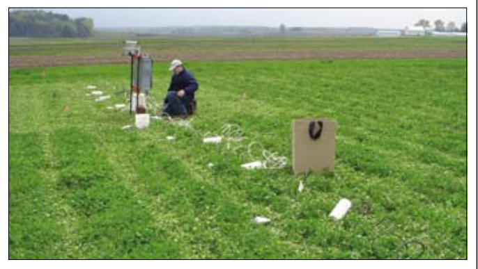
ARS technician Todd Schumacher installs soil moisture monitoring equipment in a kura clover living mulch experiment at a University of Wisconsin research farm in Arlington, Wisconsin. Row locations of recently planted no-till corn are evident from the effects of band-applied herbicide directly over the rows. (Photo by Tyson Ochsner)
