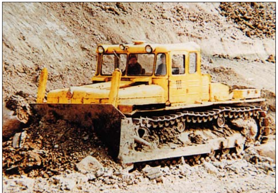
The ChTZ DET-250m2 was a massively robust dozer produced at the Cheliabinsk Works. The big machine utilised a 330 hp V12 diesel, originally designed for propelling high speed Soviet military tanks. It was but one of a vast range and assortment of track machines exported under the Belarus logo. (IMJ archives)
