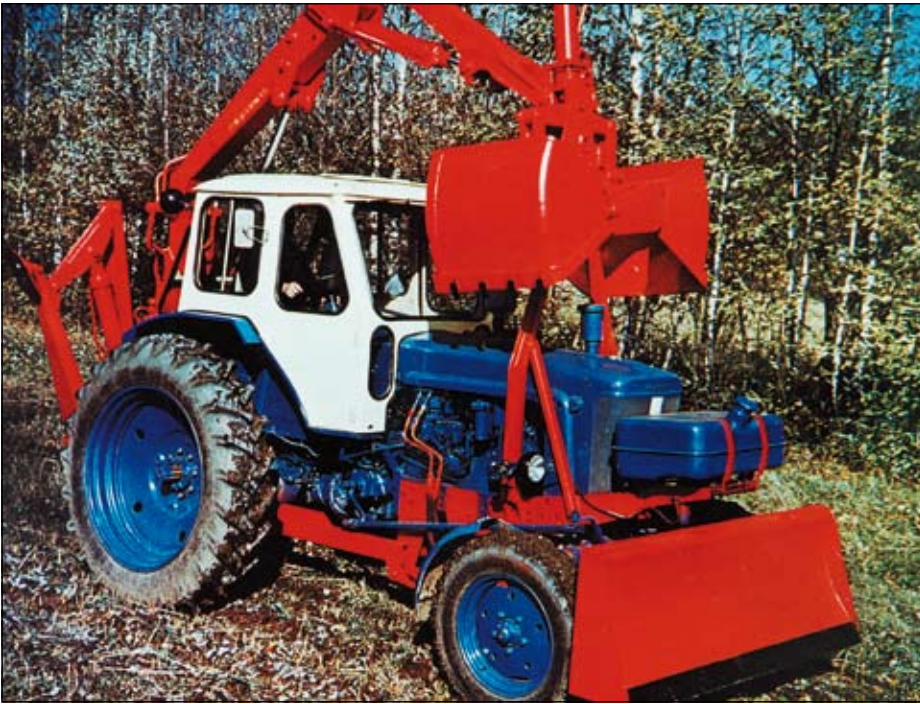
The Belarus YuMZ-6M/L pictured, was fitted with a 360° slew loader/excavator manufactured at the Agricultural Machinery Works located in the Ukrainian town of Kolomya. This super versatile machine had a lifting capacity of 800 kg when fully extended to 3.9 metres. Interestingly, the English backhoe manufacturer Whitlock Bros of Great Yeldham, produced an almost identical rig, but mounted on a Fordson Major. One example of these English machines was imported into Australia, but proved to be an engineering disaster and was abandoned. In contrast, the Belarus rig worked brilliantly and was sold in large numbers, mainly to Eastern Block countries. (IMJ archives)
