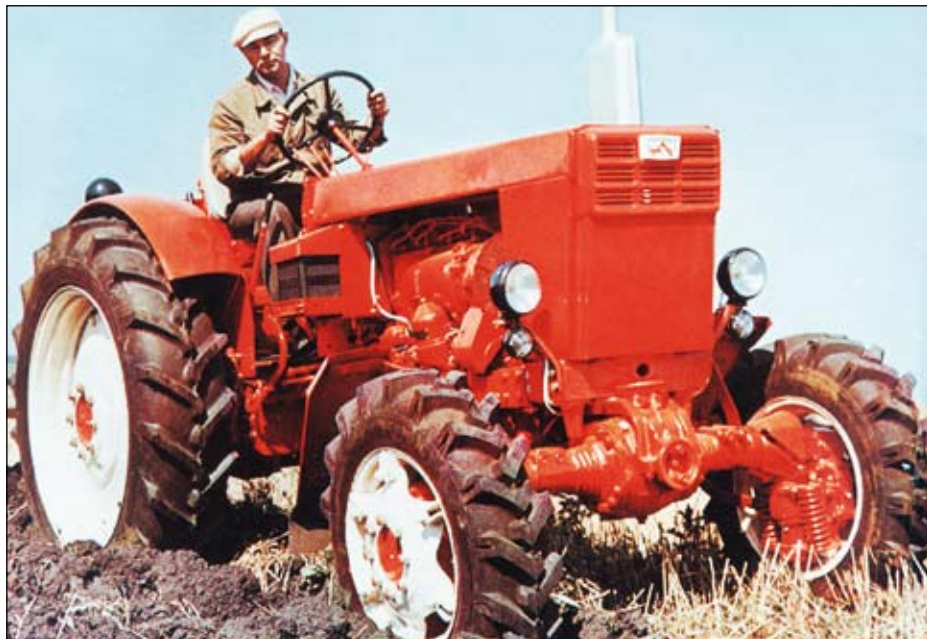
The Belarus T40 A, released in the late 1970s, featured a four cylinder air cooled diesel of 4150 cc. It was a product of the Vladimer Tractor Works. Although unwieldy in design it certainly was rugged. Note the individual front wheel suspension. (IJM archives)
